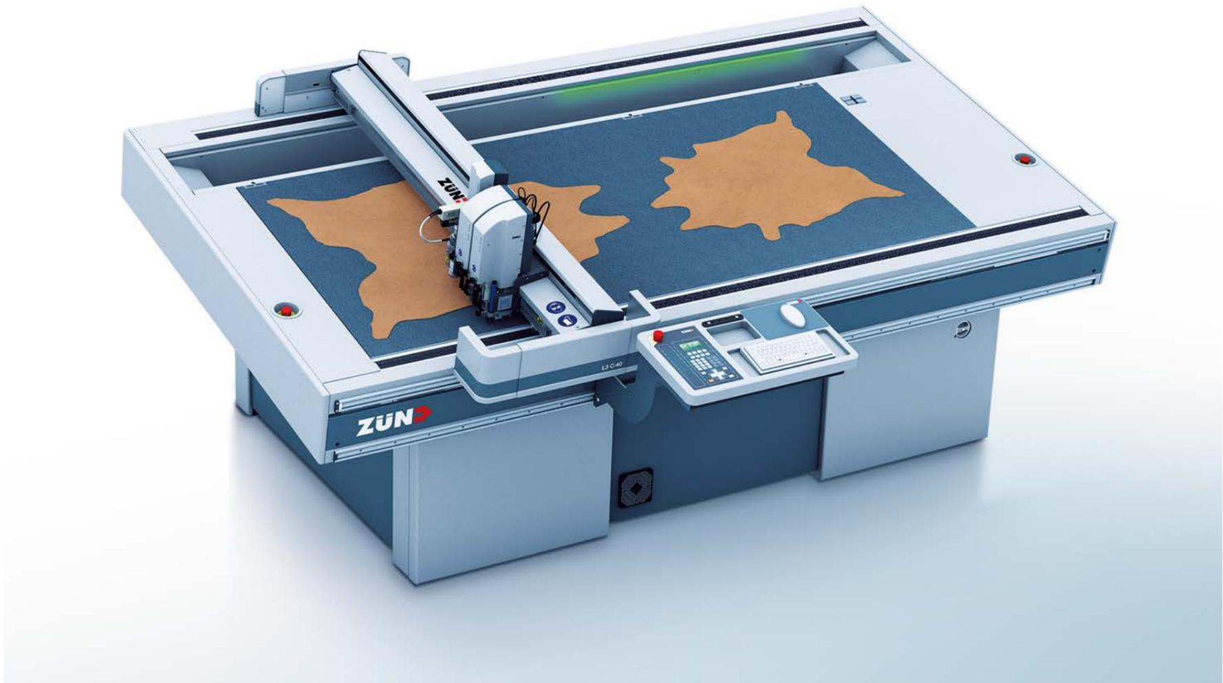
The Zünd tooling system consists of high-performance cutting, punching, and routing tools. The modularity of the system minimizes the initial cost and lets you tailor the configuration to your specific needs. The L3 can accommodate combinations of up to seven tools for different functions.
